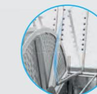
90° pivoting washing pipe with manually removable spray headers.
