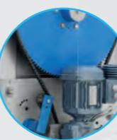
Pinion/chain/sprocket system for lower consumption.
