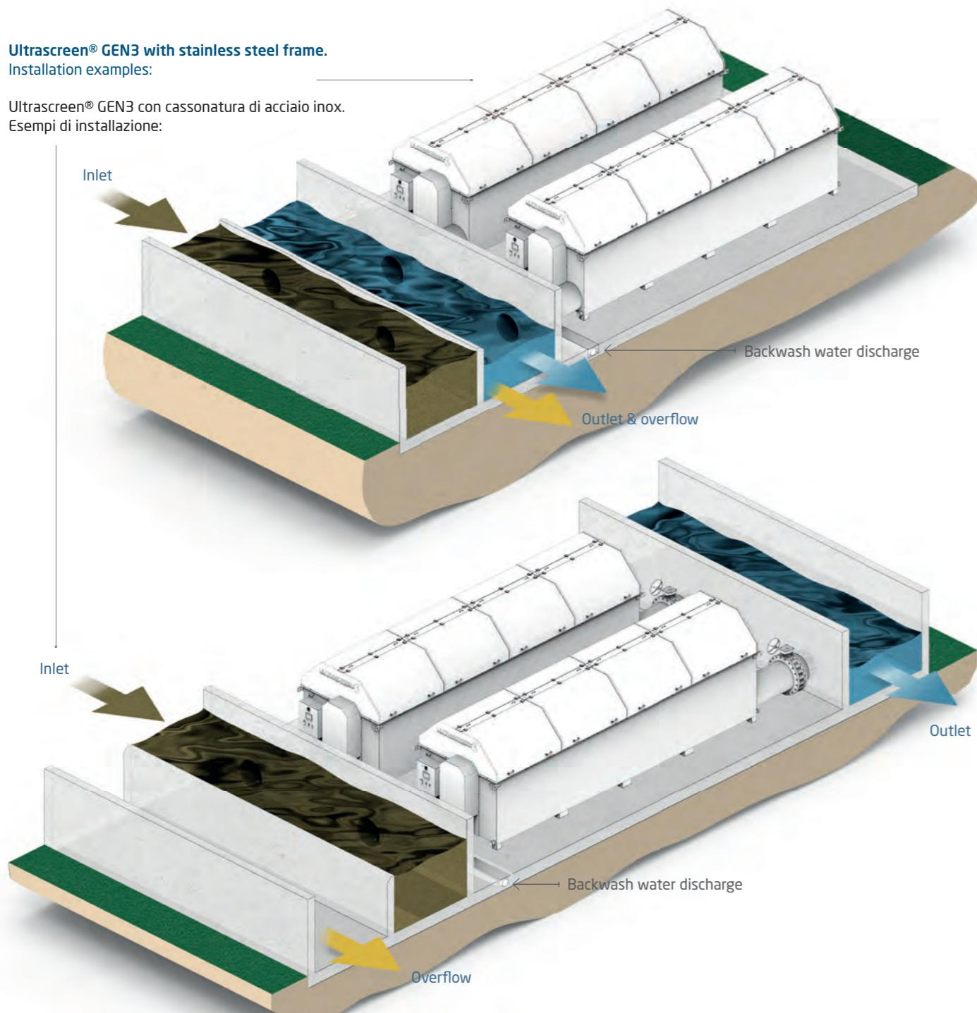
Ultrascreen® GEN3 in concrete tank.
